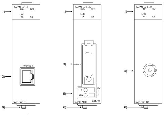
The following introduces the functions and names of parts of the FL-net module.
