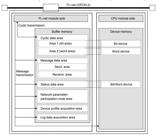
The FL-net module has a memory area corresponding to the path for each type. Exchange with the CPU module takes place through the buffer memory.
