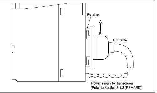
Fig. 5.1 Diagram of AUI cable connection
