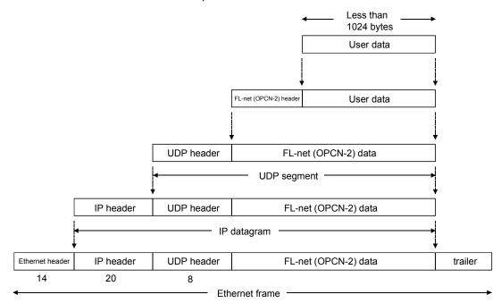
The following shows one frame of FL-net (OPCN-2) data that can be observed on a communication line.
