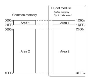
(6) Transfer methods between the cyclic data area (Area 1, 2) in the buffer memory and PLC CPU devices
