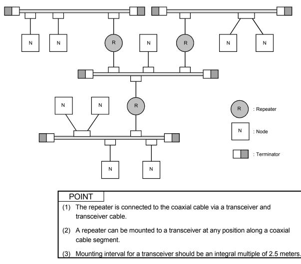
In the example in the illustration below, the maximum distance between nodes is 2,500 meters. In order to increase the transmission distance, a link cable (the maximum is 500 meters for coaxial cable) with repeaters installed at both ends is used. This is called a linked segment.
