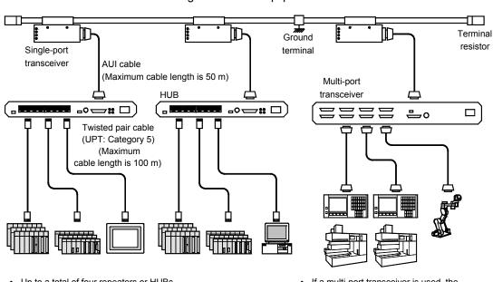
Several multi-port transceivers or HUBs are connected to one coaxial cable so that the network can consist of a large number of equipment.
