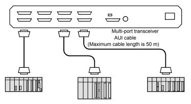
(a) When using a multi-port transceiver.
