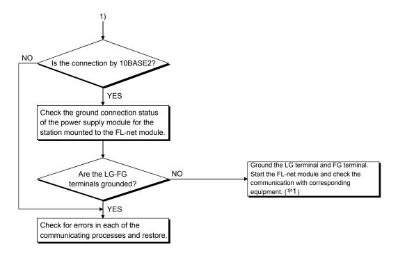
\*1 When the LG terminal and FG terminal for the power supply module for the station to which the FL-net module is mounted have not been set, the communication line may close because of noise stopping communication with corresponding equipment. Turn off the power supply to the station for the FL-net module and refer to the section on wiring in the user's manual for the CPU module for grounding terminals LG and FG on the power supply module.
