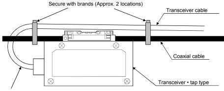
Take the bending radius of the transceiver cable into consideration (the smallest bending radius is 80 mm)
