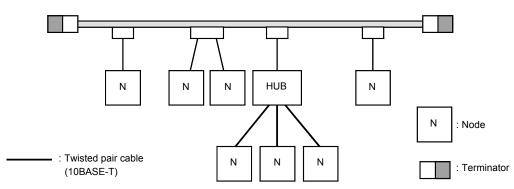
In addition, if the distance between nodes is short, the twisted pair cable can be connected to the HUB without passing through a coaxial cable or transceiver.
