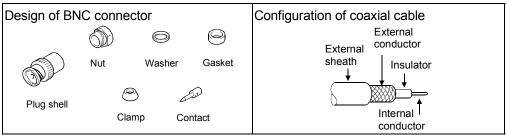
Fig. 5.4 Configuration of BNC connector and coaxial cable
